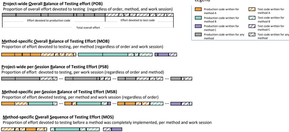
Figure 2: Measures to be derived from a programming activity event stream. Each row depicts a different method of aggregating the programming events from Figure 1.
